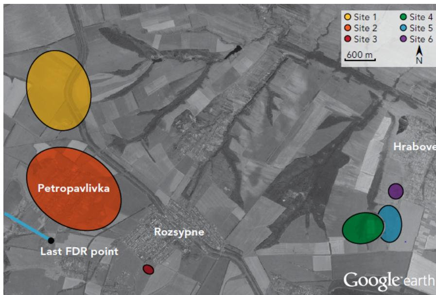
Figure 13. Overview of the six wreckage areas provided by the Dutch Safety Board. The larger areas indicate an in-flight break-up.<sup>85</sup>
