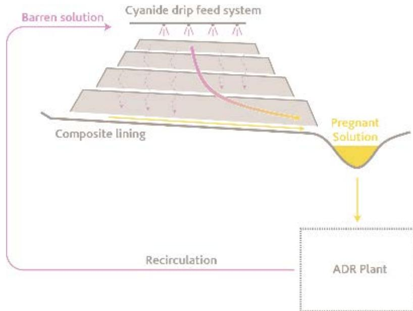
**Figure 8: Schematic of how gold is leached from the heap and how cyanide is contained by a composite lining system**
