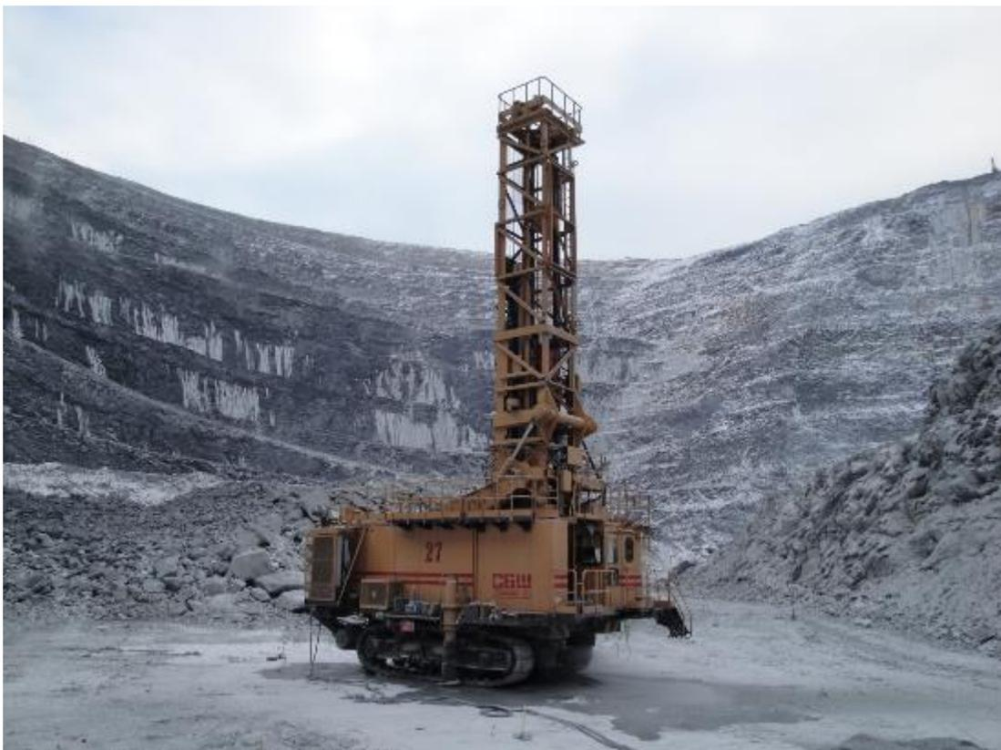
**Figure 5: Example of a drill rig in an open pit**
