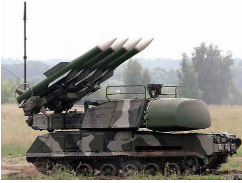
TELAR with radar 9A310
